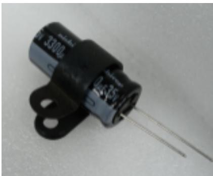
**3. Use the existing clamps to install smaller caps.** The clamp won't tighten enough to reach the diameter of the smaller cap so something must be used to fill that space. The option many use is to purchase foam that insulates pipe...glue it to the clamp and/or caps and install. It works and is cheap and easy. I prefer to use an electrical pipe spacer/reducer whenever
